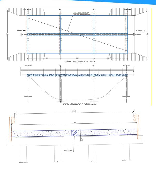
The recommended design and repair option is option 2 which will upgrade the bridge to a full SM1600 load rating and increasing the life of the bridge with the elimination of deteriorated bridge beams and use of engineered concrete components
